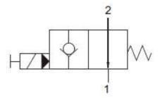
With the solenoid *switched* off the oil flows in the direction indicated by the arrows. With the solenoid *switched* on the oil flow is blocked.
